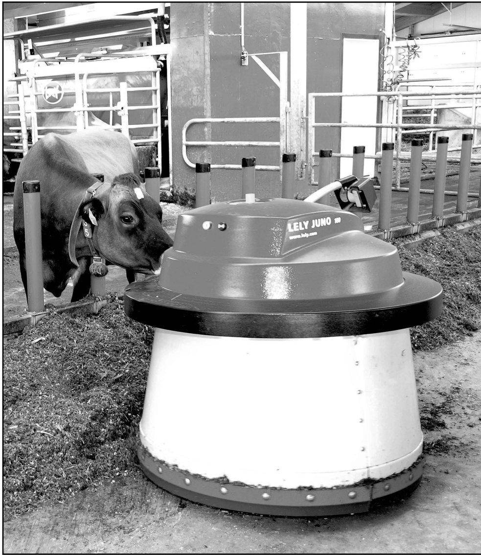
A battery-operated Juno feed pusher follows a pre-programmed route around Carnor Farms' barn, ensuring feed is always available to cows. (Staff photo by Diane Johnston)
